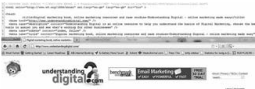
FIGURE 5.1 Screenshot showing title tag and meta-description as they appear in HTML source code, and the same page as it is rendered in the Firefox browser, showing the start of the same title tag in the active tab
